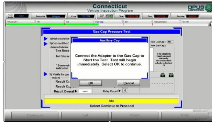
Next, the gas cap pressure test will perform a leak down test of the vehicle's gas cap. Answer all questions and proceed by clicking continue. You MUST select the appropriate response for how many tanks/gas caps the vehicle is equipped with. Vehicles with dual gas tanks MUST have both gas caps inspected. Place the gas cap on the appropriate adapter and click continue to begin the test.
