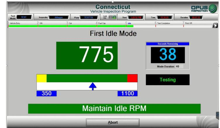
The first idle mode will measure RPM at idle. The timer will indicate the time remaining for idle mode. *\*The inspection will only require one cruise and one idle mode if the readings obtained are sufficient to deliver a result.*
