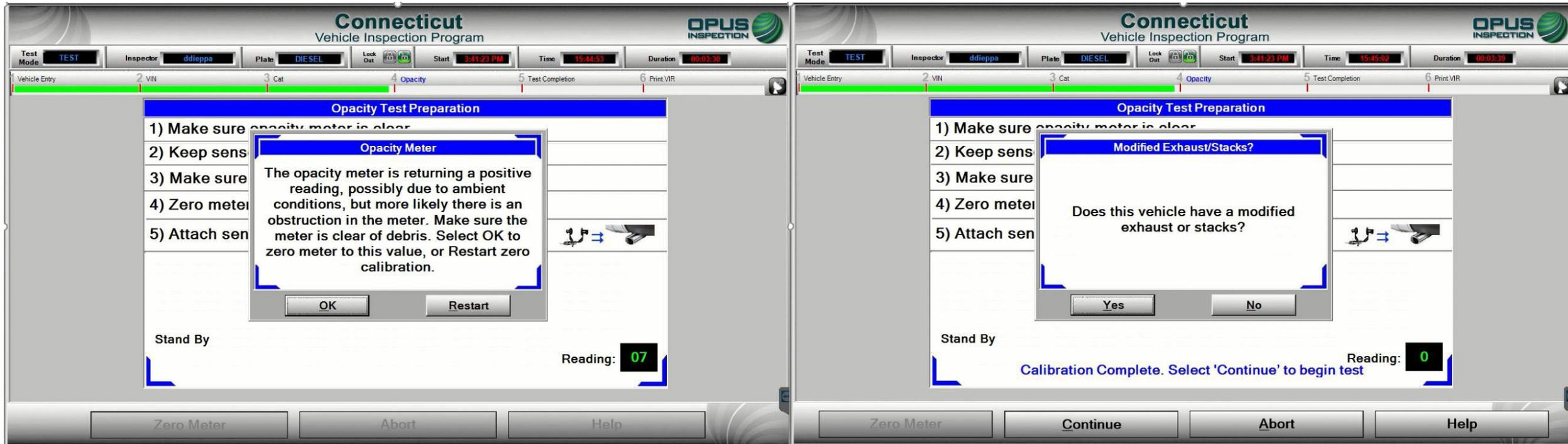
If there is an obstruction or the meter has not returned a zero result in preparation for the inspection, click OK to zero the meter. This should allow you to begin the inspection, however, you may have to exit the inspection to troubleshoot the opacity meter. Next, you will answer Yes or No to modified exhaust OR exhaust stacks.
