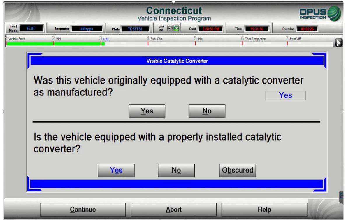
After the inspection type is determined (see above), next will be the visual catalytic converter check. Be sure to select the appropriate response, as the outcome of the test will be affected. Be SURE to perform the visual CAT check; do NOT answer without physical verification.
