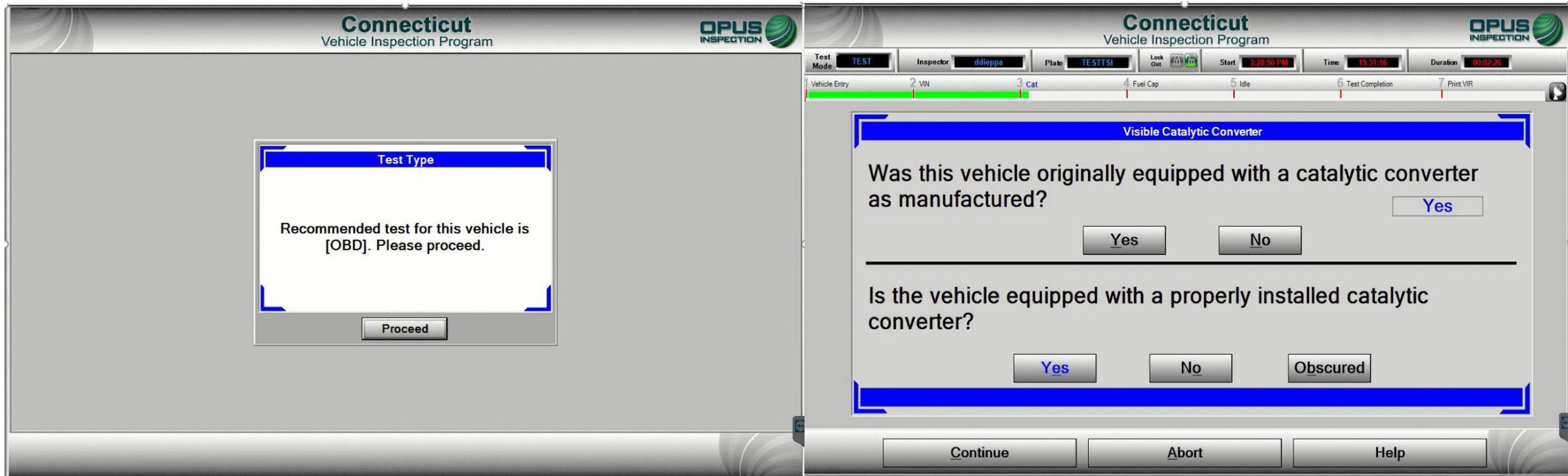
After the inspection type is determined (see above), next will be the visual catalytic converter check. Be sure to select the appropriate response, as the outcome of the test will be affected. Be SURE to perform the visual CAT check; do NOT answer without physical verification.
