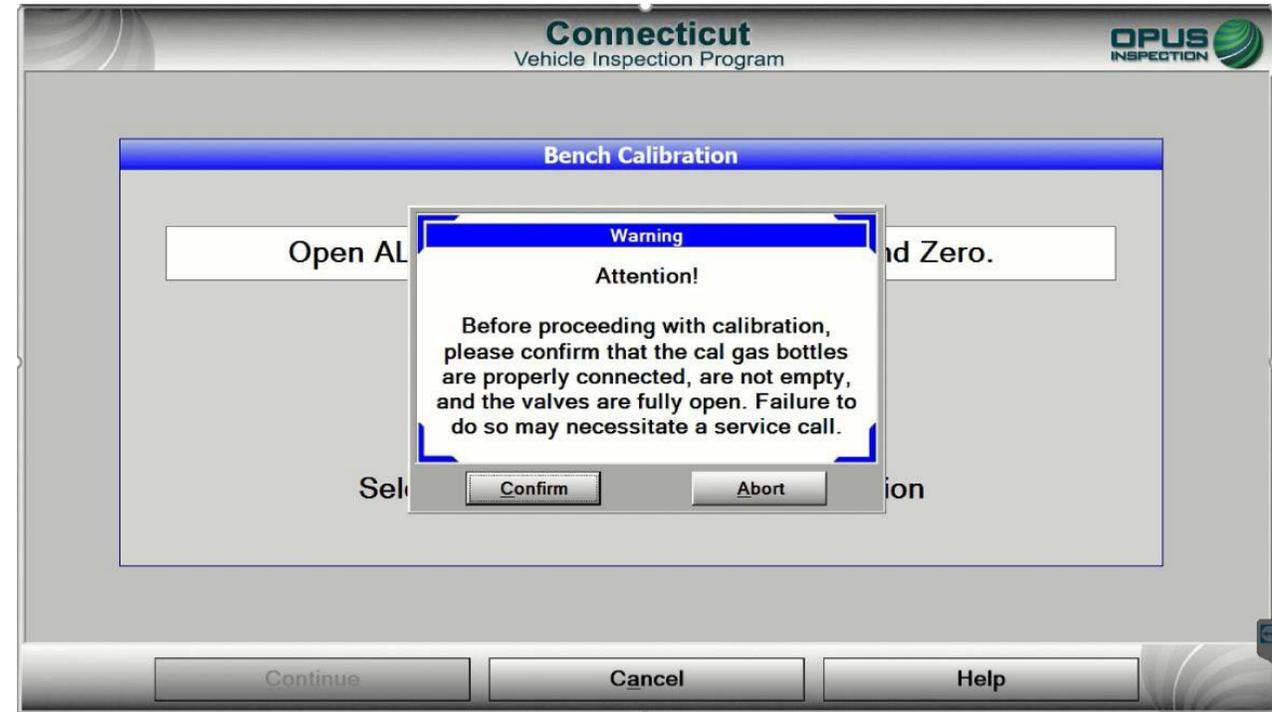
Open both High and Zero gas bottles. A warning will appear, prompting you to verify the gas bottles are properly connected, are not empty, and that the valves are fully open to ensure there are no issues with the calibration.
