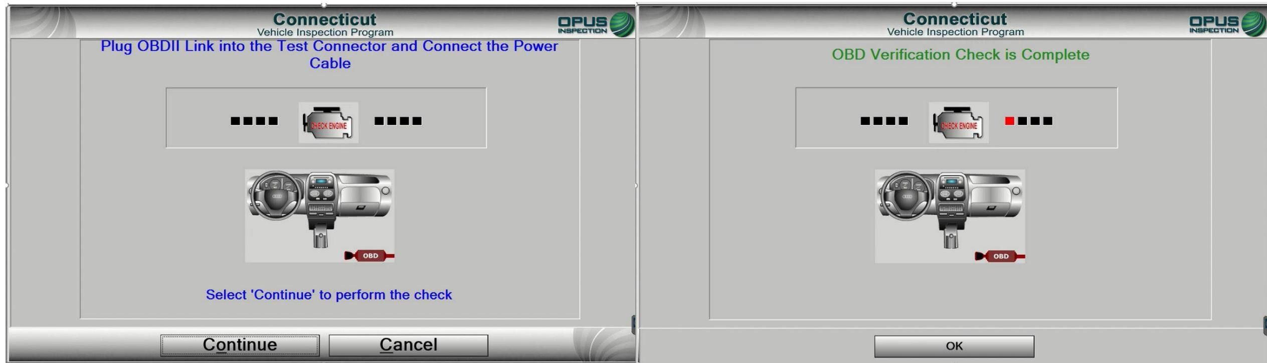
Next, connect the OBD cable to the DAD unit for a self check. The verification will complete. If there is an issue with the DAD module, check all connections and try again.
