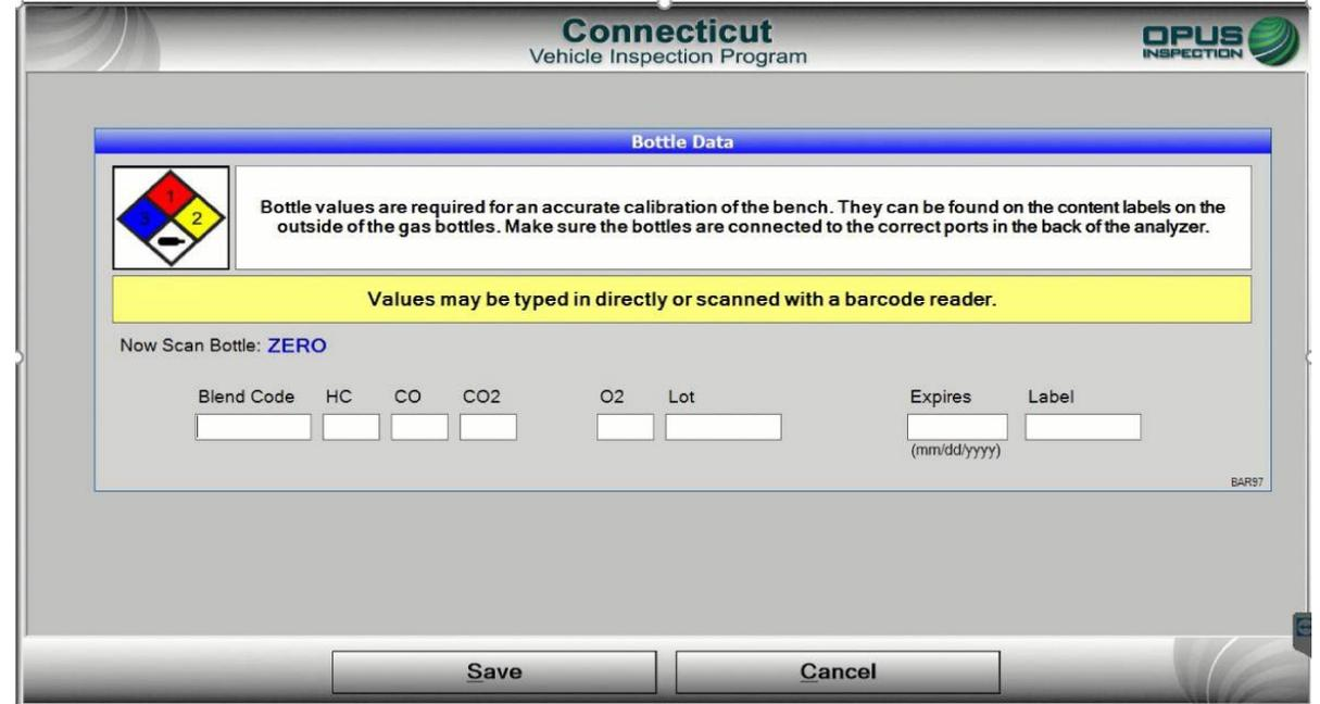
Selecting Periodic Calibration will take you immediately to Gas Calibration, which should be completed every two weeks. Scan in the barcodes from the gas bottle label. Each bottle has three barcode labels, each representing specific information; values will appear in the appropriate box when scanned and when all fields are complete, the values will be saved. If the values are already populated from a previous scan, verify the values match and continue by clicking Save.
