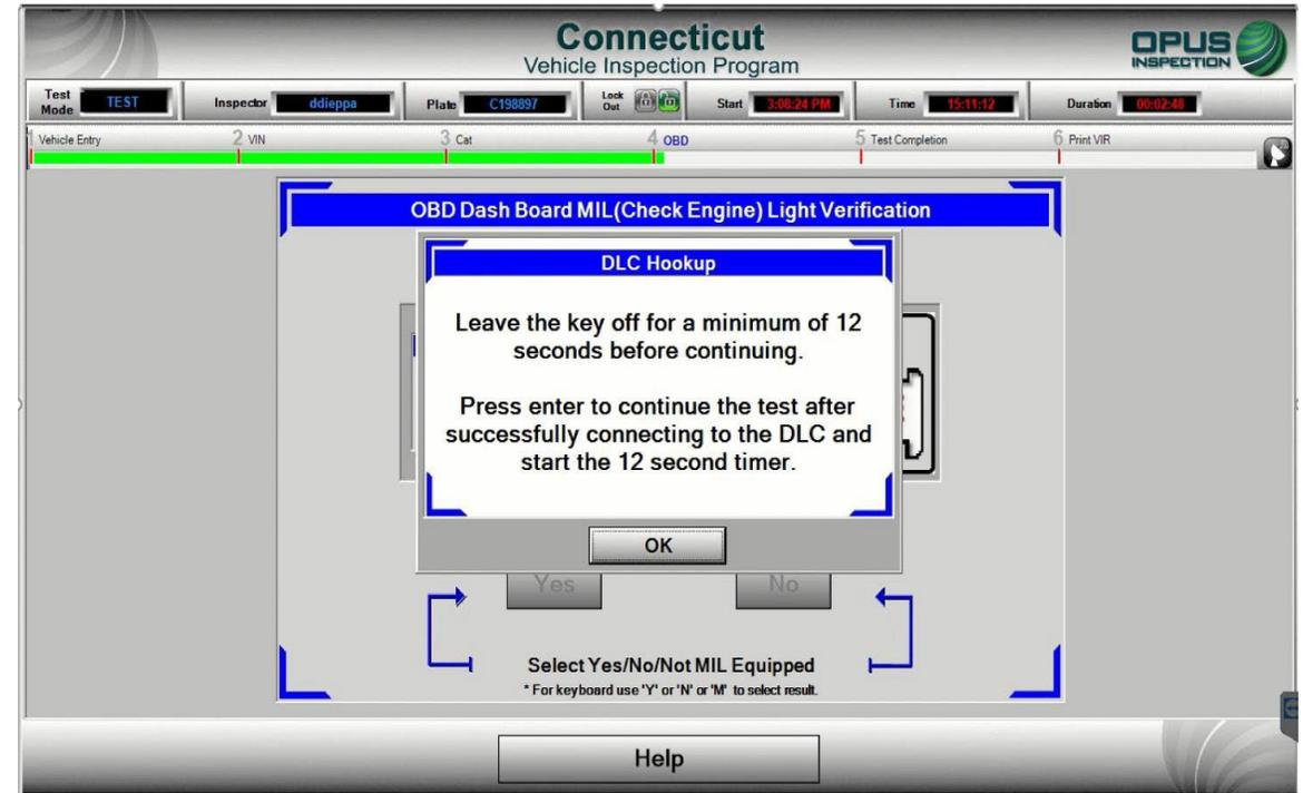
Next you will be prompted to shut the engine off and connect the OBD cable to the vehicle's DLC. You will then be prompted to verify the OBD cable is connected; upon verification, the 12-second timer will begin.
