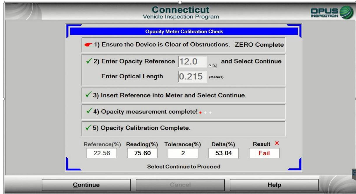
The Opacity Meter Calibration is similar to the current method, using a calibration glass to insert into the meter for readings.
