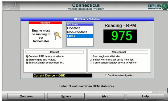
First you will capture RPM by choosing one of the methods available. You must make three attempts, using any source available before bypassing RPM. RPM bypassing is strictly monitored and bypassing without a sufficient attempt is a Program Violation subject to Monetary Assessments.
