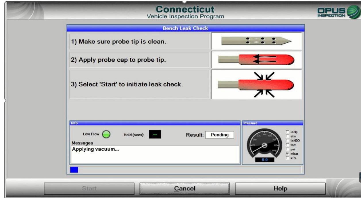
Once the calibration is complete, be sure to close the gas bottles. The leak check will be performed next; this calibration requires that only the primary hose be tested. An inspection involving a dual exhaust vehicle will prompt for a leak check of both the primary and dual hoses.
