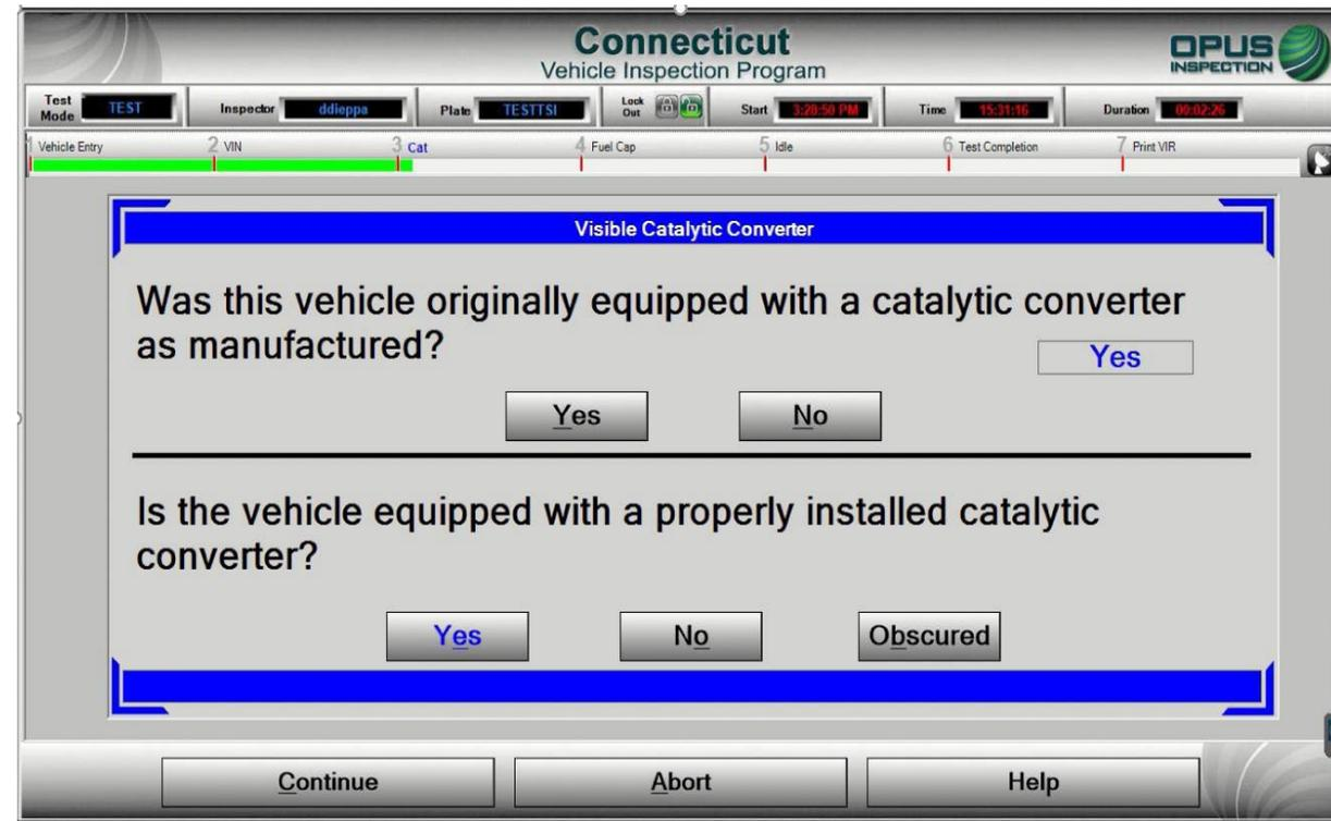
After the inspection type is determined (see above), next will be the visual catalytic converter check. Be sure to select the appropriate response, as the outcome of the test will be affected. Be SURE to perform the visual CAT check; do NOT answer without physical verification.
