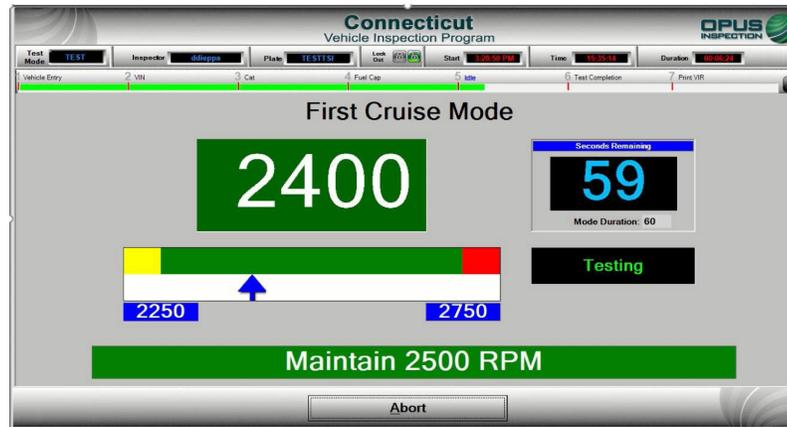
The first cruise mode will have you maintain the vehicle's RPM at 2500; the timer will indicate the time remaining for first cruise mode.
