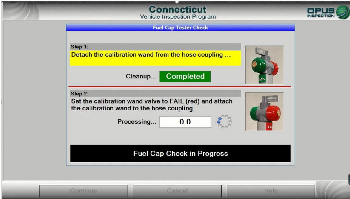
The Fuel Cap Tester Calibration has been enhanced with the Waekon calibration wand; the gas cap leak check hose connects to the bottom of the wand and the lever at the top of the wand toggles for “pass” and “fail” calibrations.
