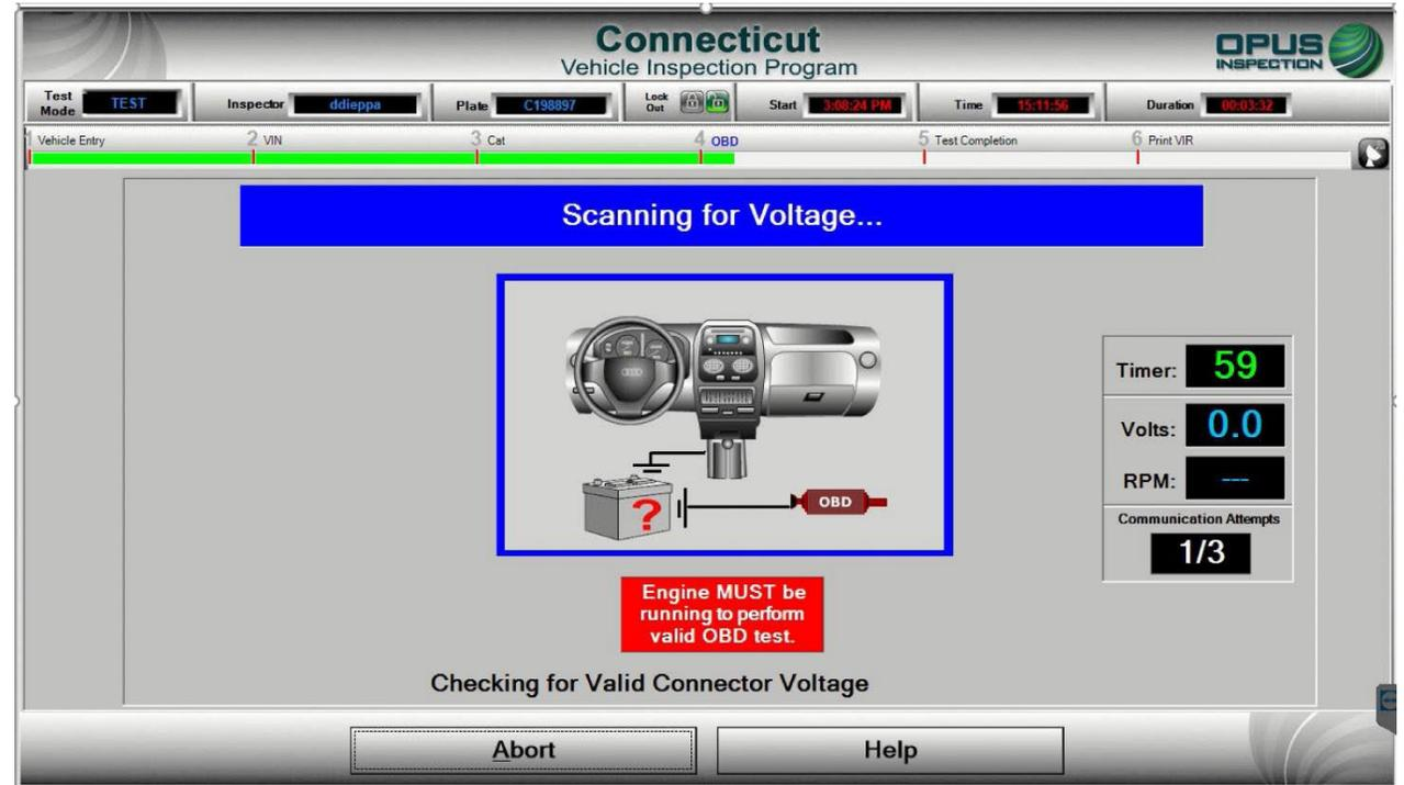
Once connected to the vehicle, the program will run through a series of protocols (above); the blue bar as shown above will display progress as the inspection continues.
