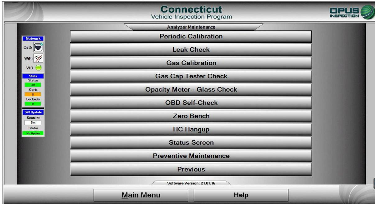
Periodic calibrations are to be performed every 72 hours. All Test Centers must be ready and able to test during program operating hours. All gas bottles have an expiration date and cannot be used once expired. Modifying the expiration dates, lot numbers, or concentration values is a program violation and is strictly prohibited.
