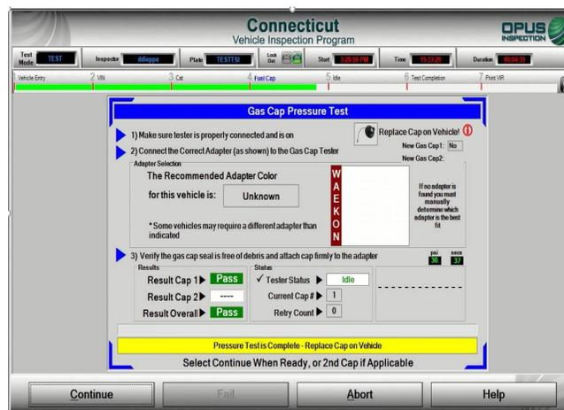
*When the test is complete, remove the gas cap from the tester, return it to the vehicle, and continue.*
