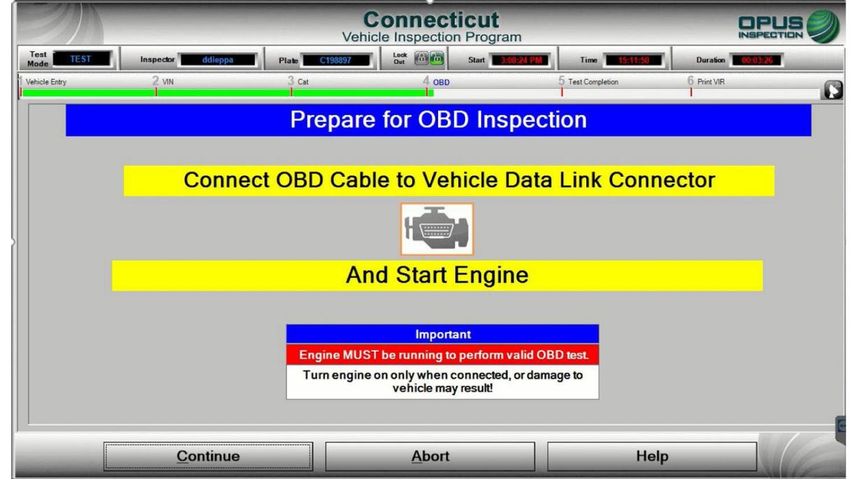
You will next be prompted to perform a Key On Engine Off (KOEO) check of the vehicle's Malfunction Indicator Lamp (MIL, also referred to as the Check Engine Light). You will then be prompted to connect the OBD cable to the vehicle's DLC. **DO NOT connect to the DLC while the vehicle's engine is running!**
