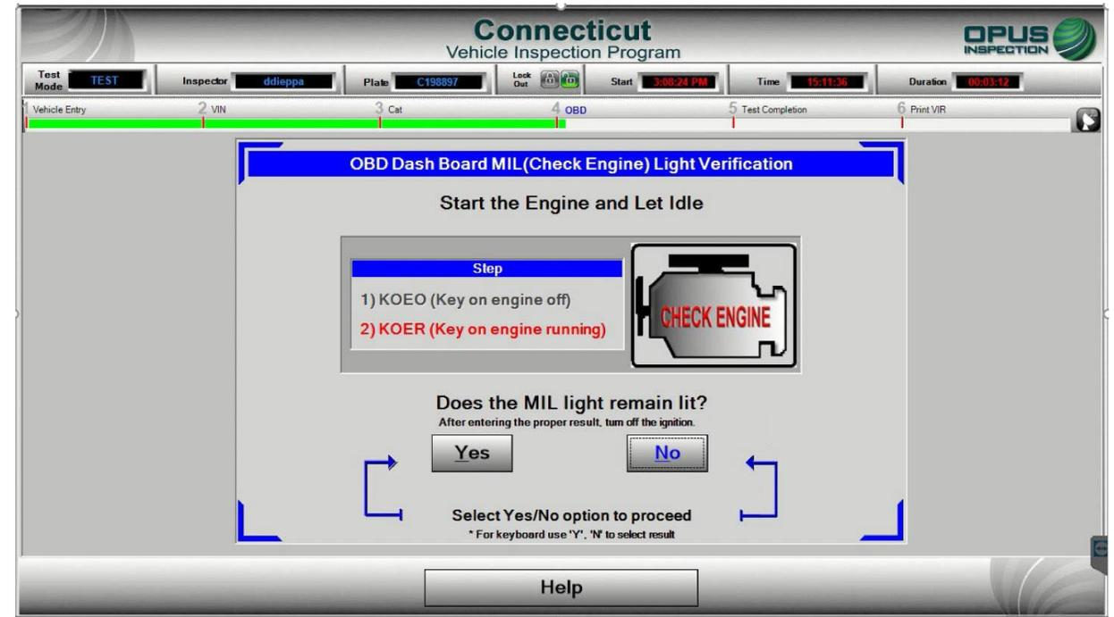
When the OBD inspection data retrieval is complete, you will be prompted to turn the engine **OFF** and disconnect the OBD cable from the vehicle's DLC. Next, perform a Key On Engine Running (KOER) check to confirm that the MIL light does not remain illuminated while the engine is running. The inspection is now complete.
